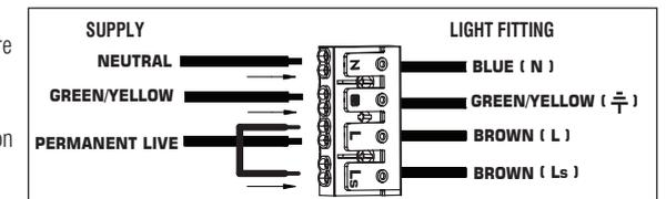
**Maintained (Switched) Wiring:** The product is used as a normal light - switch on/off, light turns on/off. Comes on during a power failure.
